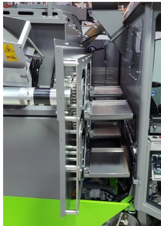
Stainless Steel Tracking Plate with 5 off Stainless Steel Crate Trays
